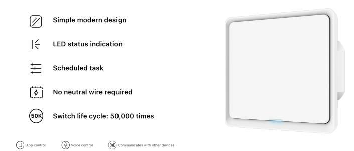
General ESW-1ZBC-EU Model: Platform : Tuya In-wall concealed with 86 back box Installation L in, L out Wiring: -5~45°c Operating Temperature: Operating Humidity: 5~90% Power Supply: AC 100-240V 50/60Hz Maximum Overload: LED: 5-300W per channel incandescent: 3-300W per channel Control Unit: 16A magnetic latching relay Switch Life Cycle 50,000 times Indicator Light: Yes
