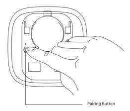
**Note:** Press and hold the button for 12 seconds to enter pairing mode. The LED will flash rapidly.
