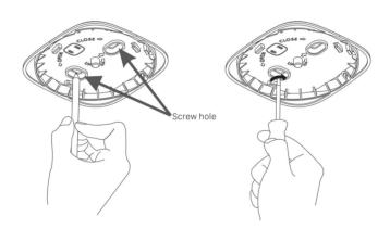
Align the body of the product with the "Product Installation Icon" marked on the bracket. Gently rotate the product body clockwise until you hear a distinct "click" sound. This confirms that the product is securely locked into the bracket.
